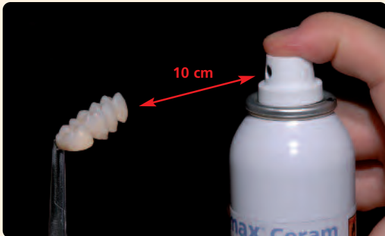
Observe a distance of 10 cm when applying the IPS e.max Ceram Glaze Spray.
