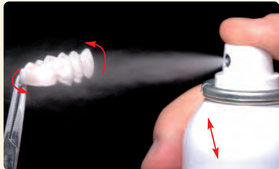
Spray IPS e.max Ceram Glaze Spray with short bursts directly on the unfired Essence materials and/or Shades from different directions.
