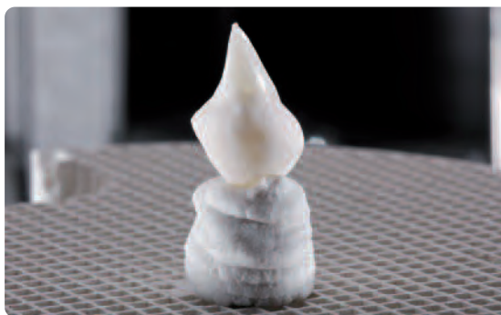
Place the abutment on a honey-combed firing tray for the Dentin firing.
