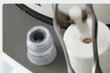
Then, place the powder-coated IPS Alox Plunger into the hot investment ring.
