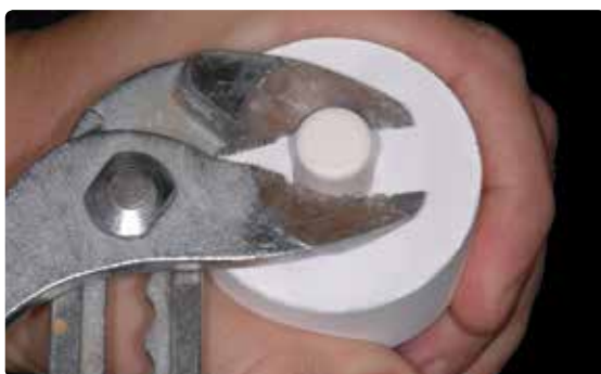
The Alox plunger is already very clean if it is removed with tongs from the investment material. Check the cleanness and blast with Al_2O_3 , if required.
