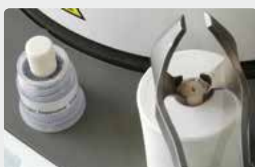
Insert the cold IPS InLine PoM ingot with the imprint facing upwards into the hot investment ring.
