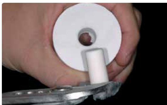
The Alox plunger is already very clean if it is removed with tongs from the investment material. Check the cleanness and blast with Al_2O_3 , if required.
