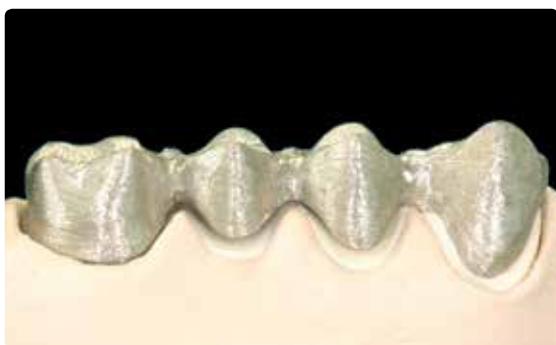
Surface finishing before blasting.
