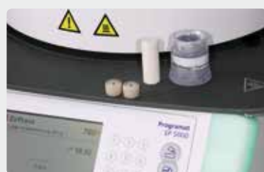
Provide a cold IPS Alox Plunger and cold IPS InLine PoM ingots in the desired shade.
