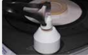
Place the cold IPS One-Way plunger 300 g in the hot investment ring.
