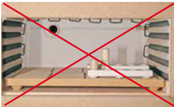
Do not preheat the IPS InLine PoM ingots and the IPS One-Way plunger/AloX plunger.
