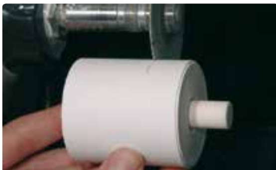
Separate the investment ring using a separating disc.
