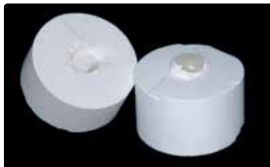
Separate the investment ring using a separating disc.
