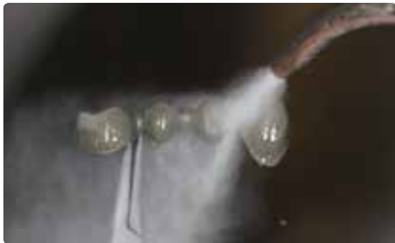
After blasting, clean the metal framework with a steam jet and allow to dry thoroughly. Conduct the oxide firing according to the instructions of the manufacturer.
