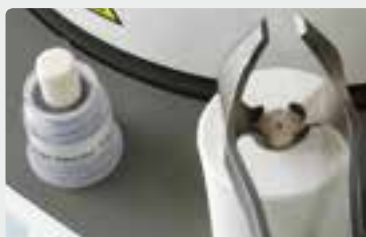
Insert the cold IPS InLine PoM ingot with the imprint facing upwards into the hot investment ring.
