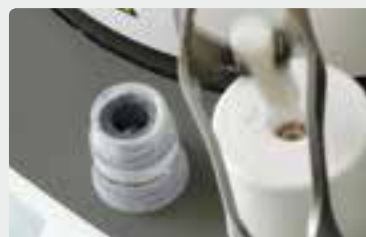
Then, place the powder-coated IPS Alox plunger into the hot investment ring.
