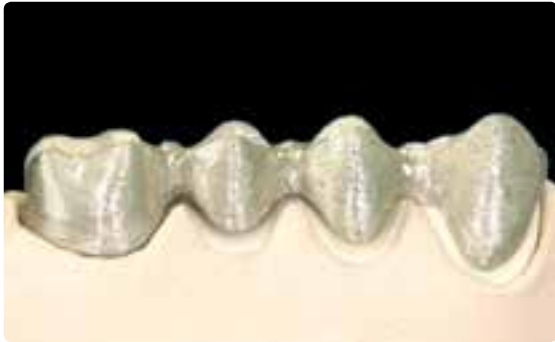
Surface finishing before blasting.
