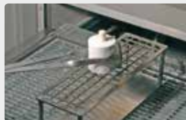
Once the press program is completed, place the hot investment ring on the cooling grid using the investment ring tongs and allow it to cool to room temperature.
