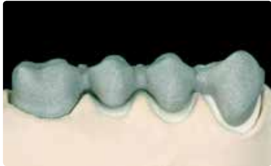
Carefully blast the framework with aluminium oxide Al_2O_3 , 50–100 \mu m (observe the instructions of the alloy manufacturer).
