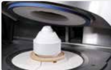
Place the hot and completed investment ring in the centre of the hot press furnace using the IPS Investment Ring Tongs.
